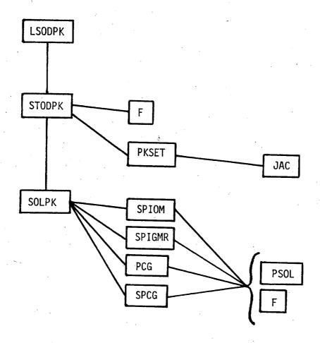
Fig. 1. Simplified Block Structure of LSODPK
