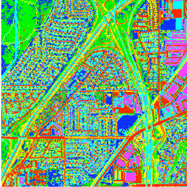
Figure 11: Image B classified using k-means algorithm, with 6 classes. Original satellite image by Space Imaging.
