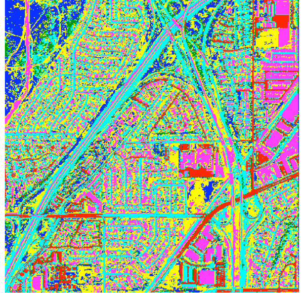
Figure 12: Image B classified by a decision tree algorithm using 4860 pixels from Figure 7. Original satellite image by Space Imaging.
