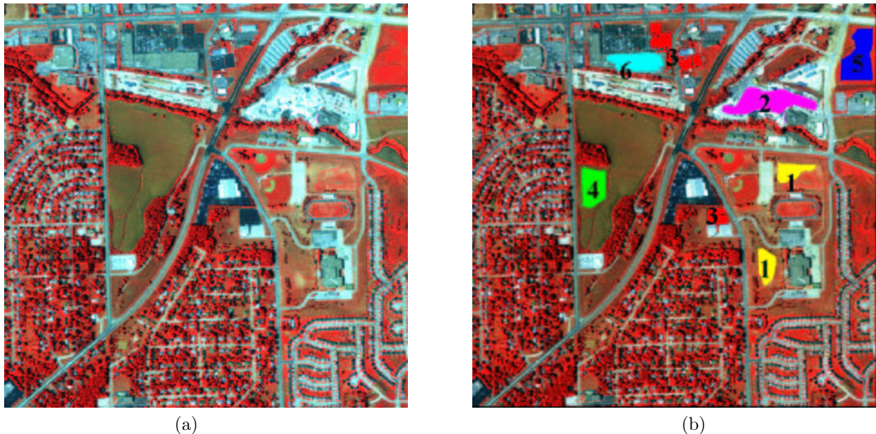
Figure 1. (a) A 400 \times 400 pixel multi-spectral image from Nebraska. (b) The regions in the image from which pixels were chosen for the 6 classes. Satellite images by Space Imaging.
